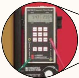
Blower Door tests help diagnose and detect air leakage problems and estimate efficiency losses because of the leakage. The Digital Gauge, pictured above, measures and displays building pressure.
